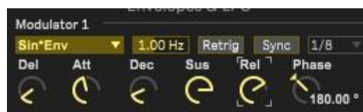
Fig. 28 Example of Modulator 1 settings; here the amplitude of the sine LFO is modulated by the ADSR envelope
