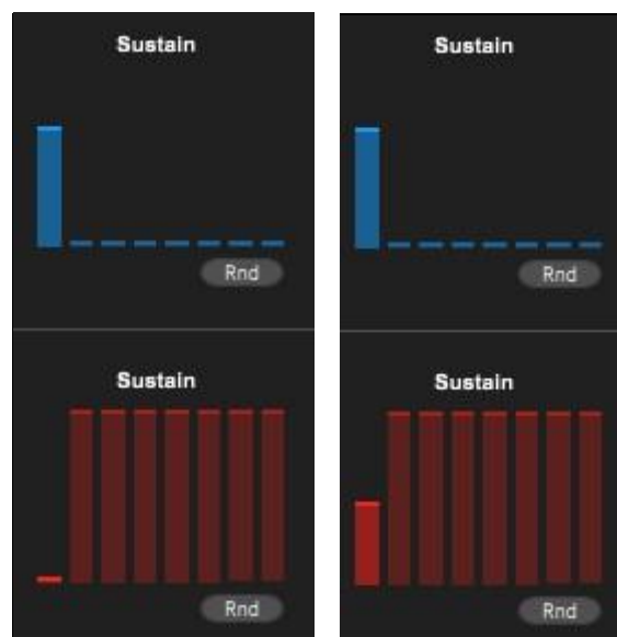
Fig. 13 Setting the FM Sustain levels for the first partial: on the left a sine wave can be heard, on the right the Frequency Modulation is active
