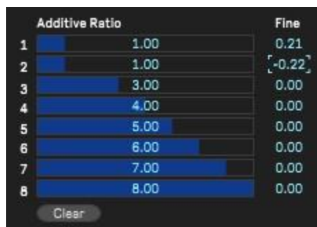
Fig. 9 Setting the frequency ratio for each part in the Expert Parameters section of the Edit window
