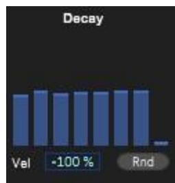
Fig. 12 Using the Random function and the action of velocity on Decay times
